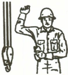
TRAVEL. (One Side Track). Lock the track on side indicated by raised fist. Travel opposite track indicated by circular motion of other fist, rotated vertically in front of body (for land cranes only).
