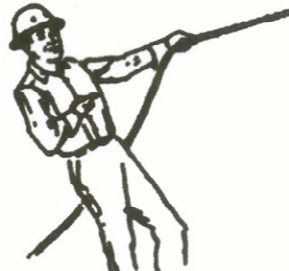
RETRACT BOOM (Telescoping Boom). One-hand signal. Hold one fist in front of chest, thumb pointing outward and heel of fist tapping chest.
