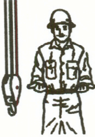
EXTEND BOOM. (Telescoping Booms). Hold both fists in front of body, thumbs pointing outward.
